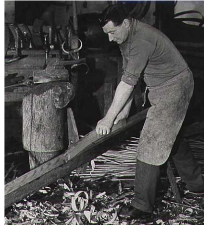
2. Smoothing stave edges with the 'jointer' GDB/DB06/0005.09
