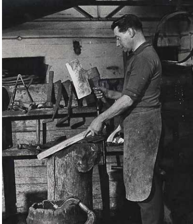
1. Roughly shaping the stave with the 'axe' GDB/DB06/0005.06
