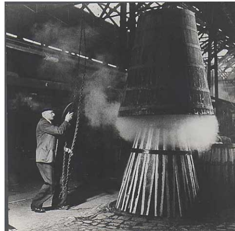
4. 'Steam bell' being lowered over the cask GDB/BR14/0003.14
