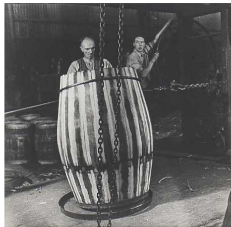
6. Bending the stave ends together GDB/BR14/0003.17
