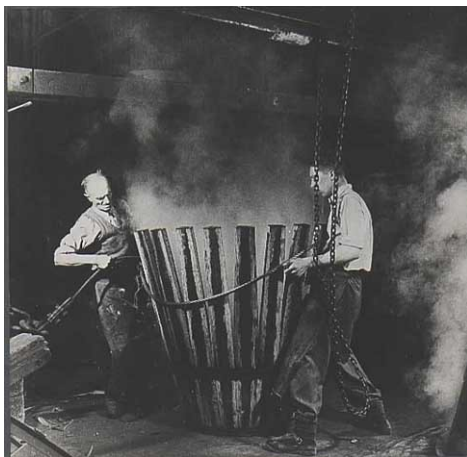
5. Placing the rope over the stave ends GDB/BR14/0003.15
